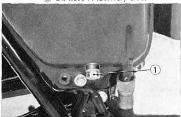
Fig. 15-7 ① Oil tank drain plug
