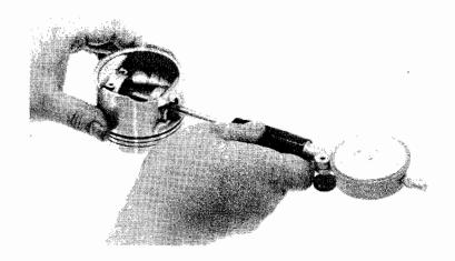
Measure the connecting rod small end I.D. (See Section 12 for replacement procedure)
