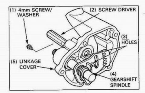
Install the linkage cover/gearshift spdindle assembly with the screwdriver through the hole in the shifter. Install and tighten the gearshift linkage cover bolts.
