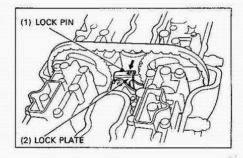
Install the cam chain guide.
