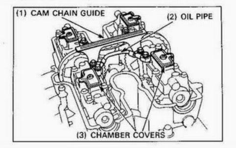
Loosen the cam chain by pushing the cam chain tensioner lock pin down and pulling the lock plate up until the lock plate resets on the lock pin shoulder as shown.
