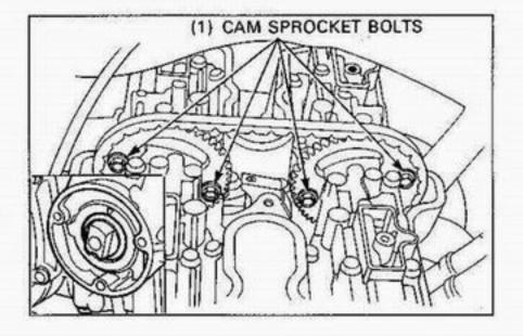
Remove the cam sprockets from camshaft flange with the cam chain.
