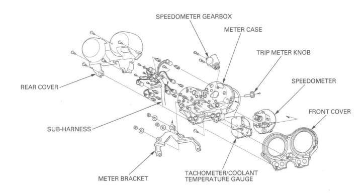
Assemble the combination meter in the reverse order of removal.
