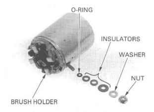
Push and hold the brush inside the brush holder. and install the armature through the brush holder. When installing the armature into the motor case, hold the armature tightly to keep the magnet from pulling the armature against the motor case.
