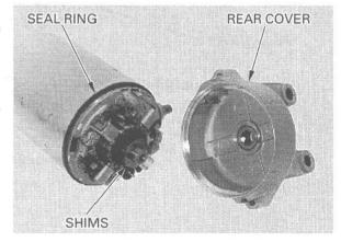
Install the shims properly as noted during removal.
