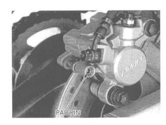
Install and tighten the pad pin plug.
