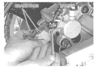
Always replace the brake pads in paris to assure even disc pressure.
