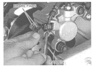
Install and tighten the pad pin.
