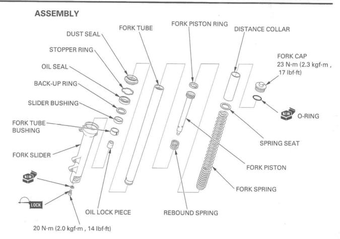
Before assembly, wash all parts with a high flash or non-flammable solvent and wipe them dry.
