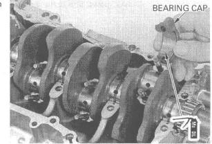
Apply oil to the connecting rod nut threads and seating surfaces.
