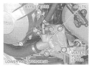
Remove the O-ring from the water pump body. Remove the water hose from the water pump body. Remove the water pump body from the crankcase.
