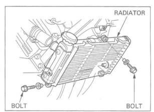
Connect the lower radiator hose and tighten the hose clamp screw securely.
