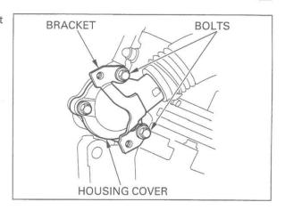
Install the thermostat housing protector and tighten the two bolts.
