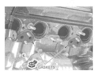
Install the secondary air supply tubes to the cylinder head, tighten the four nuts securely.
