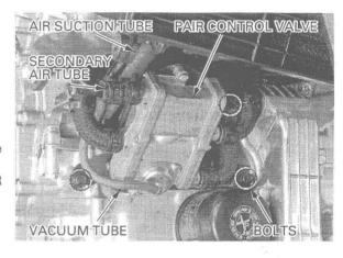
Remove the nuts and secondary air tubes from the cylinder head.
