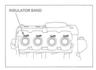
Tighten the insulator band screws so that the band ends clearance is 10  $\pm$  1 mm (0.4  $\pm$  0.04 in).
