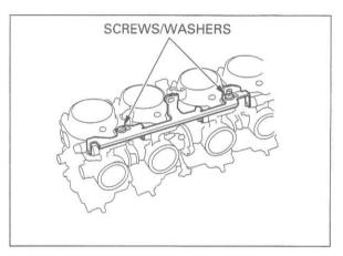
If the throttle sensor is removed, install the throttle sensor aligning its boss with the groove on the throttle shaft plate.
