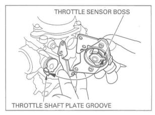
Install and tighten the throttle sensor bracket mounting screws.
