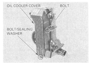
Remove the bolts, washers and oil cooler. Remove the O-rings and joint collars from the oil cooler base.
