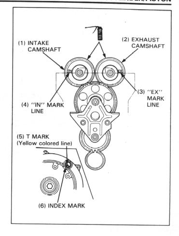
Install the dowel pins onto the camshaft holders and install the camshaft holders in their original positions.
