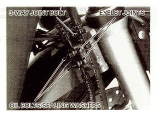
Remove the brake pipe joint nut.
