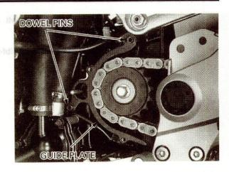
Install the drive sprocket cover and tighten the SH bolts.
