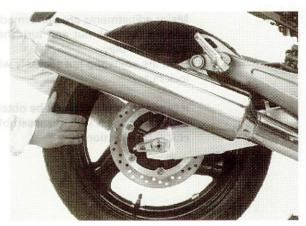
Check for worn swingarm bearings by grabbing the rear swingarm and attempting to move the swingarm side to side.
