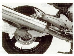
Check the action of the shock absorber by compressing it several times.
