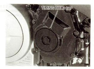
Turn the crankshaft clockwise, align the "T" mark on the ignition pulse generator rotor with the index mark on the ignition pulse generator rotor cover.
