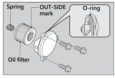
**9.** Install the oil filter cover by tightening the oil filter cover bolts.
