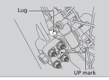
3. Tighten the front axle shaft.
