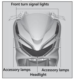
The headlight/front turn signal lights/ accessory lamps use several LEDs. If there is an LED which is not turned on, see your dealer for servicing.
