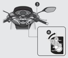
**5** Press the start button with the throttle completely closed. Release the start button as soon as the engine starts.
