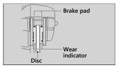
**1.** Inspect the brake pads from underneath the brake caliper.
