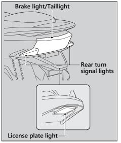
The brake light/taillight/rear turn signal lights/license plate light use several LEDs. If there is a LED which is not turned on, see your dealer for servicing.
