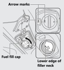
Do not fill with fuel above the lower edge of the filler neck.
