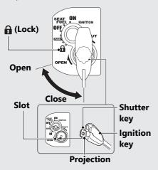
The shutter will automatically close when you remove the ignition key at the (Lock) position.
