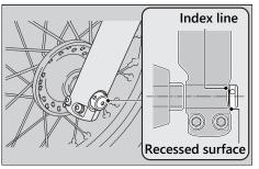
4. Tighten the left axle pinch bolts.
