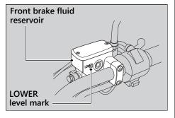
If the brake fluid level in the reservoir is below the LOWER level mark or the brake lever freeplay becomes excessive, inspect the brake pads for wear.
