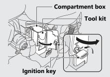
Insert the ignition key and turn it counterclockwise to unlock.
