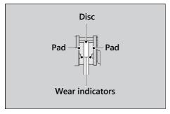
Inspect the brake pads from the bottom of the brake caliper.
