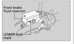
If the brake fluid level in the reservoir is below the LOWER level mark or the brake lever freeplay becomes excessive, inspect the brake pads for wear. If the brake pads are not worn, you most likely have a leak. Have your motorcycle inspected by your dealer.
