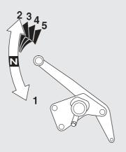
If you put the motorcycle in gear with the side stand down, the engine will shut off.
