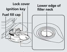
Do not fill with fuel above the lower edge of the filler neck.
