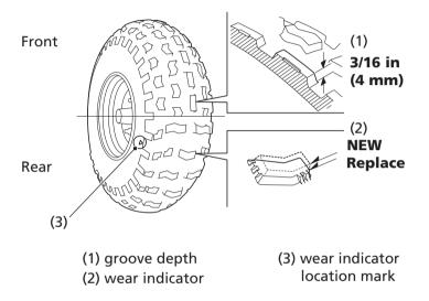
To check the condition of a tire tread, measure the groove depth (1) in the center of the tire, or check the wear indicator (2). For best performance, you should replace a tire before the tread depth at the center reaches the following limits:
