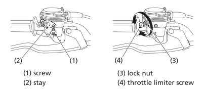
For higher top speed, removing the air intake restrictor is required. Adjusting for increased throttle lever movement without removing the air intake restrictor will cause the engine to run roughly at higher speeds.
