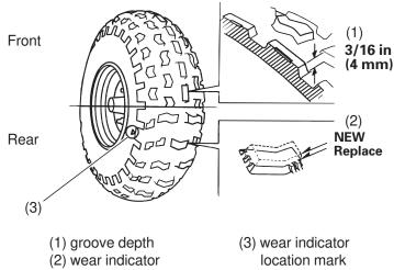
To check the condition of a tire tread, measure the groove depth (1) in
