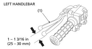
(1) rear brake lever/parking brake lever
