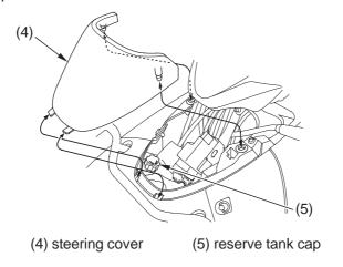
5. After adding coolant, install the reserve tank cap and steering cover.
