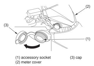
The accessory socket (1) is attached to the right side of the meter cover (2). You can use the accessory socket to power a trouble light, spotlight, CB radio, or cell phone, etc.
