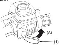
(1) throttle lever(A) to open the throttle
