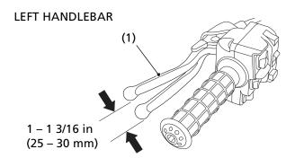
(1) rear brake lever/parking brake lever
