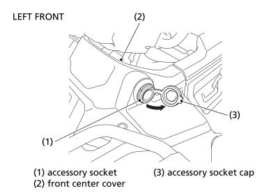
The accessory socket (1) is attached to the left side of the front center cover (2). You can use the accessory socket to power a trouble light, spotlight, CB radio, or cell phone, etc.
