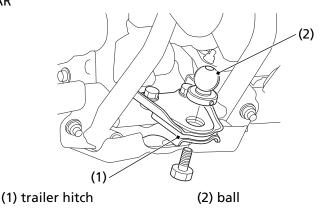
The trailer hitch (1) is located on the rear frame. To use the hitch, you'll need a proper size ball (2) as specified by the trailer manufacturer.
