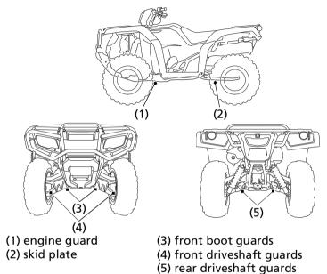
The engine guard (1) protects the engine crankcase. The skid plate (2) protects the frame.
