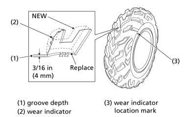
To check the condition of a tire tread, measure the groove depth (1) in the center of the tire, or check the wear indicator (2). For best performance, you should replace a tire before the tread depth at the center reaches the following limits:
