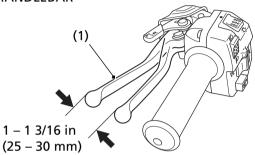
(1) rear brake lever/parking brake lever
